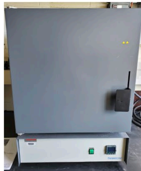
CBBs are cured at 100° C for 1 h
