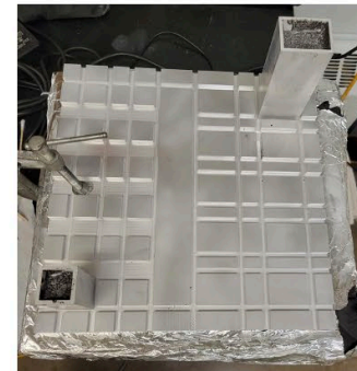
Mixture is poured into molds and vibrated to remove bubbles
