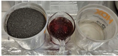
Weighed anthracite, hardener & resin/modifier
