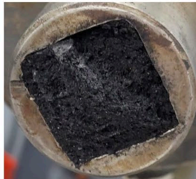
Homogeneous mixture is extruded, cut, and cooled
