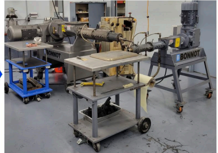
Barrel and nozzle are preheated according to transition temperatures
