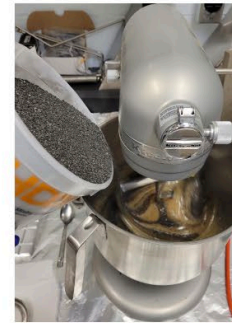
Anthracite is added to epoxy system
