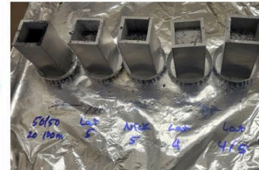
Molds are filled and compacted
