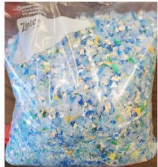
Virgin or post-consumer re-cycled (PCR) plastic binder
