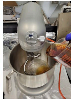
Hardener is added to premixed resin/modifier
