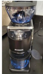
Plastic is ground to <math><850\text{ }\mu\text{m}</math>
