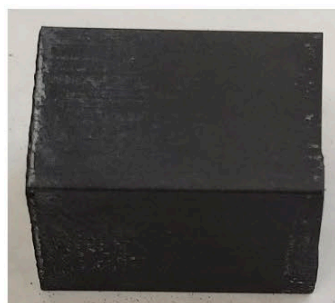
Brick is decoupled from mold
