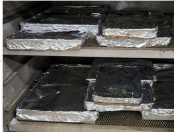
Pans are loaded into convection oven to remove moisture
